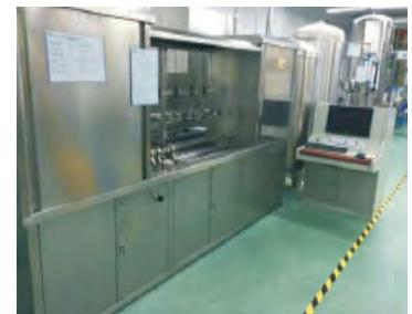
**ECO** WATER METER TEST BENCH
